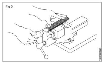
For removing the local uneveness draw filing can also be done (Fig 6). The same filing can also be done for fine finishing start filing by pushing the fine uniformly during the forward stroke and release the pressure during the return stroke.
