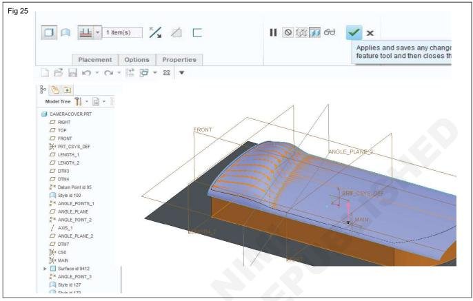
**Step 28:** Draw the circle with ø 40 mm sketch on the top plane. Extrude the sketch to about 12mm extrude
