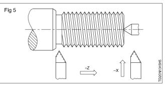
For every 3 depths of cuts by the cross-slide, give one axial cut by feeding the tool axially for 5 divisions of the compound slide. This relieves the load on the tool. (Fig 6)
