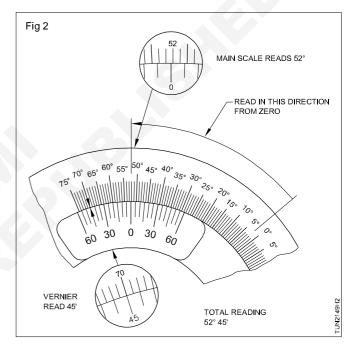
Read the vernier scale with reference to the main scale.
