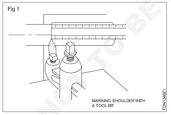
Rough and finish turn the diameter to within about 1 mm of the required length.
