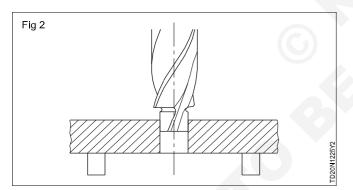
Reaming drilled holes using hand reamers
