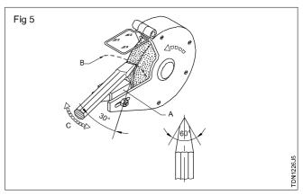
Dip the chisel in the coolant as and when it is required so as to avoid overheating.
