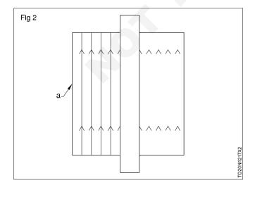
If there are two reference planes on the job, use a steel rule and working from the reference plane 'a' mark the measurements once. (Fig 3)
