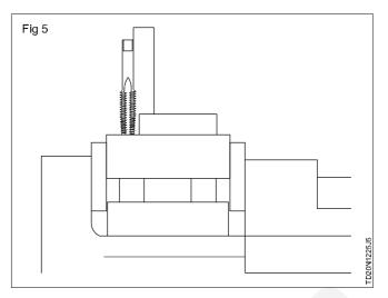
Make correction if necessary by exerting slightly more pressure on the opposite side of the tap inclination.
