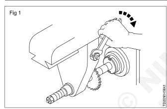
The use of a key may result in the breakage of the slitting saw if it gets jammed into the cut during cutting.
