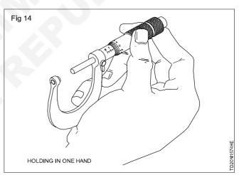
Hold the outside micrometer in your right hand, keeping the graduations on the main scale towards you.
