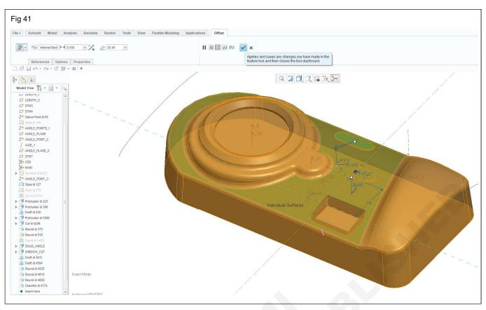
**Step 42:** Select the shell option under references tab select the removed surface surf 24, surface 33, surface
