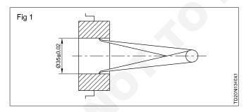
If the 'feel' is hard, reduce the distance between the leg tips and if the feel is less or if there is no feel, increase the distance between the leg tips slightly.
