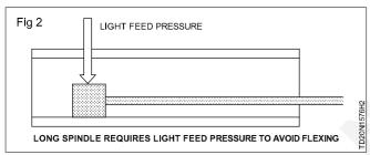
For setting up the internal grinding spindle of a universal grinding machine, the general procedure is as follows:
