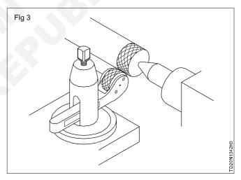
Do not feed the knurl on the work before starting the machine to avoid damage of the knurls.
