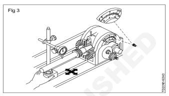
Disengage the worm from the worm-wheel for rapid indexing.
