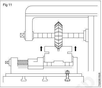
Start the machine spindle and mill the 'V' groove. (Fig 12)
