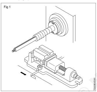
Insert enough spacers on to the arbor so that the last spacer extends over the rear edge of the workpiece. This will enable you to fix the cutter in the middle of the workpiece for milling. (Fig 2)
