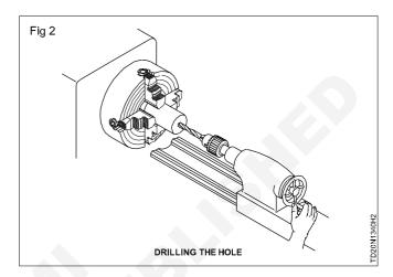
Apply cutting fluid and drill the hole to the required depth.
