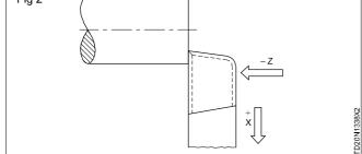
Position the tool tip near the edge of the work. (Fig 3)
