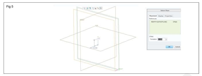
**Step 11:** Once again select the plane option in the datum tab, In datum plane dialogue box, placement tab reference select the front plane & give offset translation value to 30.00 & then select ok option. (DTM 3)
