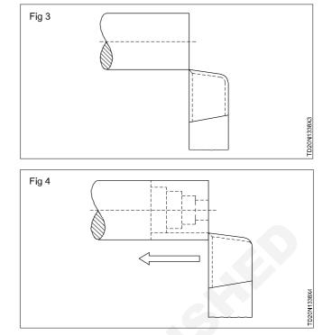
Restrict the depth of cut to a maximum of 3 mm for each cut.
