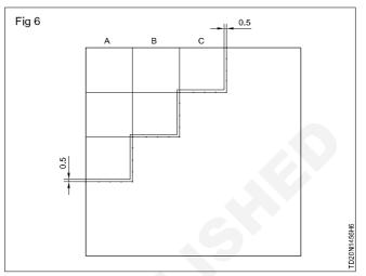
Leave 0.5 mm allowance of material on both the axes for the final finish.
