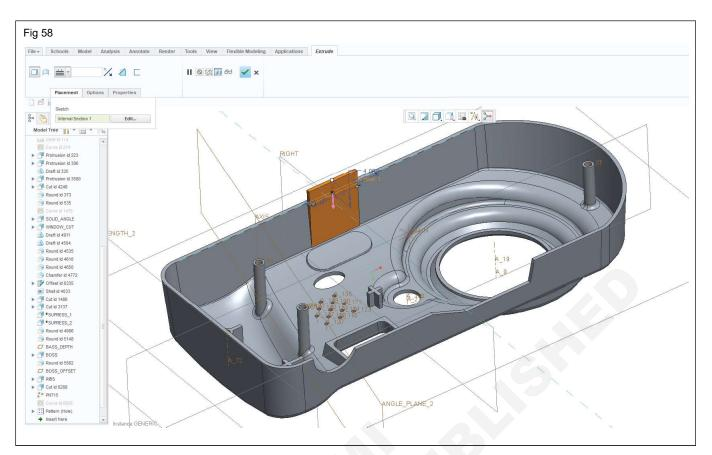
**Step 57:** Select intent surface i.e (4 faces) (as draft surface), In Pull direction select the top surfaces & give the angle as 10. (Fig 60)
