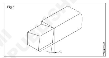
Grind the front clearance angle of 6°. Angle  $\alpha_n$  (Fig 6)
