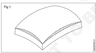
Check the flatness with a straight edge and locate the lowest spot by visual examination.
