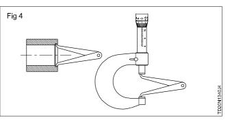
Calculate the amount of material to be removed from the hole for the roughing cut.
