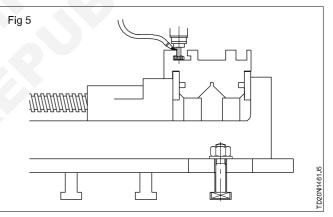
Ensure that the table movement is gentle and smooth to avoid damage to the cutter.
