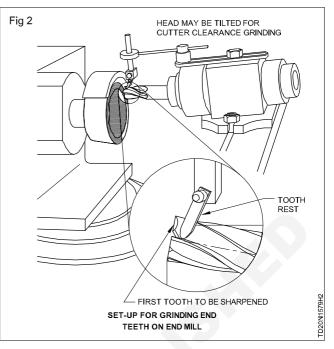
• Set the first tooth on the tooth rest, parallel to the top surface of the table (Fig 3)
