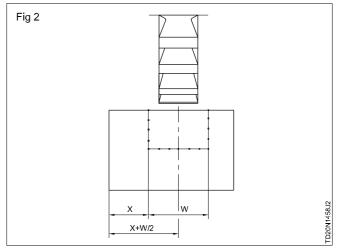
Set the depth of cut taking reference from the top surface of the job.
