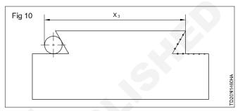
Adjust the cross-slide to get the correct calculated dimension.
