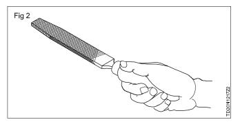
Hold the tip of the file according to the quantity of the metal to be removed.
