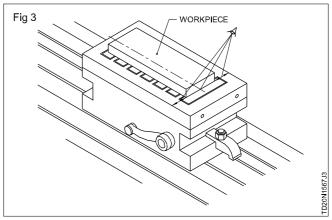
Mount the workpiece on the magnetic chuck, (Fig 5) resting the lengthier surface with the side stopper plate of the magnetic chuck.
