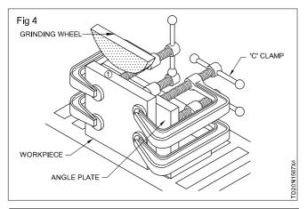
Carefully fasten two more clamps, on the end of the workpiece to hold the work securely.
