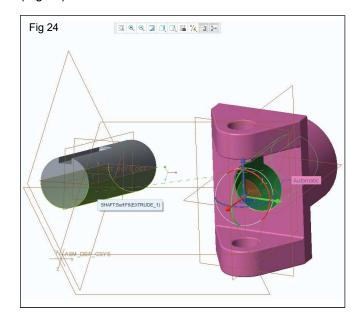
**Step 6:** Flip constraint options are used if the components needs to be flipped as per our required direction.
