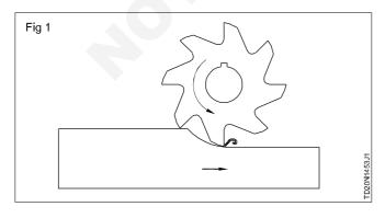
causes a good deal of heat and wear on the cutter. As the cutter teeth emerge from the material, the accumulated cutting forces are suddenly released.
