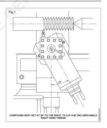
The angle to which the compound rest is set affects the cutting action of the cutting tool by producing a shearing action on the trailing edge of the tool. This produces a smooth cut.
