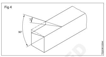
Grind the side clearance angle of 6°. Angle a (Fig 5)
