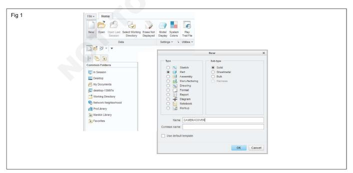
**Step 5:** In name box enter a name for the model as camera cover
