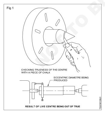
(A run out in live centre will cause misalignment during resetting the work between centres.)
