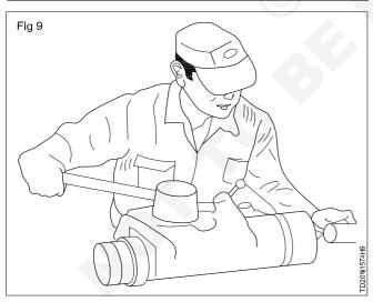
Where the tailstock centre has a nut for adjusting nut so as to allow the work to be turned lightly by the fingers.
