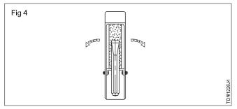
Keep the pressure as minimum as possible to prevent excessive heating of the cutting edges, (avoid blue colour i.e annealing effect) Rock the point on both sides in an arc to provide convexity at the cutting edge. (Fig 5) See the arrows 'C' separate pare.
