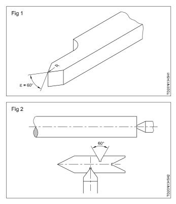
Ensure that the top slide is set at 0°, and slackness is removed by gib adjustment.
