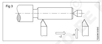
Bring the tool to the starting point and engage the half nut.
