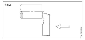
Feed the tool about 0.5 mm by the top slide inside the face of the work. (Fig 3)
