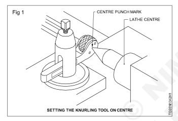
Set the machine for a low speed, preferably 1/3 to 1/4 of the turning speed.
