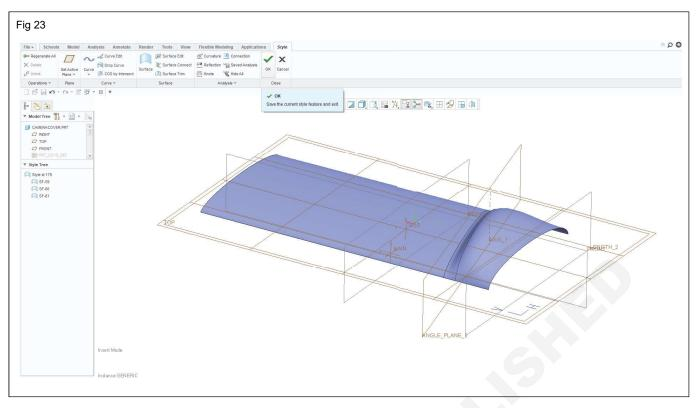
**Step 26:** In the face of rectangular surface created previously, create a sketch as per the given dimension in (Fig 24) (or) as with rough dimension.
