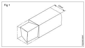
The side cutting edge is in line with the blank edge and the end cutting edge is inclined at an angle of  $25^{\circ}$ . The side rake angle is  $14^{\circ}$ . The front and side clearances are ground  $6^{\circ}$ . The length of the side cutting edge is maintained equal to the size of the square cross-section of the tool blank, i.e. 12 mm. Fig 2 shows the shaded portion to be removed by grinding the tool blank to get the ground tool. The procedure in sequence is as follows.
