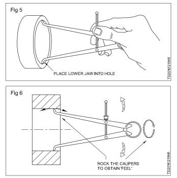
When a satisfactory sense of 'feel' is felt, transfer the measurement over a steel rule or precision measuring instrument as the case may be.
