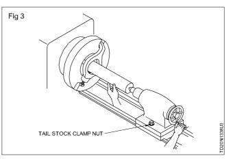
Ensure the tailstock spindle is away from the face of the work by 60 to 100mm.
