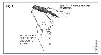
Each symbol must be made with a single blow. A second blow gives a distorted second impression.
