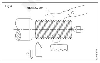
Check with the pitch gauge to confirm the gear box setting. (Fig 4)
