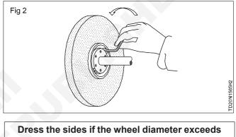
250mm. Apply a small in feed of the diamond until eccentricity of the wheel is removed.
