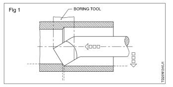
Mount the boring tool on the tool post of the compound rest.
