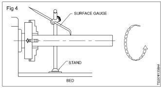
Rotate the chuck by hand and observe the gap between the pointer and work surface for the position of the two opposite jaws.
