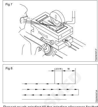
Repeat rough grinding till the grinding allowance for that side is ground away.
