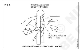
Lift the drill off the wheel face. Retain the grip on the drill with the right hand.
