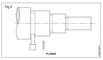
Stop the lathe and check the undercut for its dimensions. Remove sharp corners, if any.
