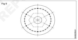
The hexagon is shown in the centre with a dotted line. To index from one side to the adjacent side, the crank is rotated to
