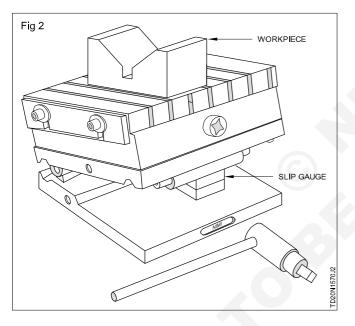
Clean the job and measure it to determine the grinding allowance. (Ask your instructor for help in determining the allowance).
