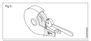
Caution; If any abnormal sound is noticed, stop the machine. Cracked or improperly balanced wheels are dangerous.
