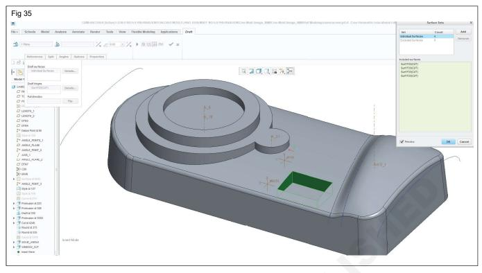
**Step 36:** As the above steps select the extruded feature face. In reference tab under draft surface details – Select faces as shown in Fig 36 under draft hinges select top &
