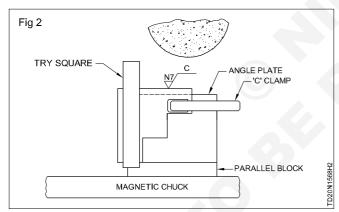
• Ensure that the surface (c) is 1 to 2 mm above the top surface of the angle plate.
