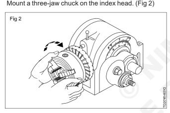
Hold the job in the three-jaw chuck at the index head and lock it.
