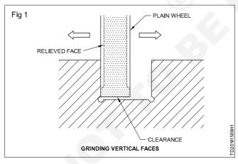
Dress the wheel for the faces, clean up and relieve both sides of the wheel if a straight wheel is used.
