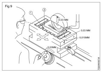
Stop all traverses and turn off the coolant. Position the workpiece away from the wheel.
