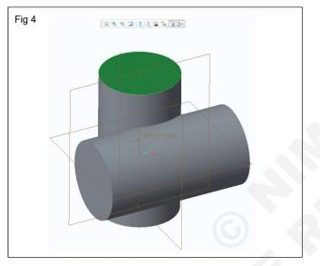
Draw circle with dia. of 16 mm on the faces of extrude to create circular holes as shown in Fig 5.
