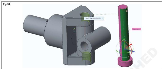
**Step 17:** Select the outside face of holding arm of fork & pin head bottom face to coincide constrain in component
