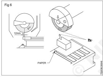
• The point of the diamond should be offset about 12mm from the grinding wheel centre line with reference to the direction of rotation of grinding wheel (Fig 6)
