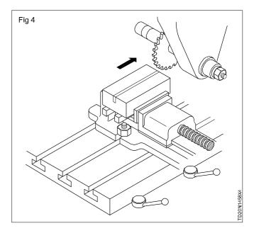
By moving the vertical slide upward, apply a depth of cut. (Fig 5)
