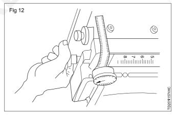
Fix the upper table do trial grinding to repeat adjustments for obtaining the given taper.
