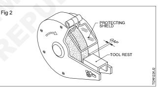
**During grinding :** Take a blunt chisel for re-grinding. Chisel will become blunt due to use. For efficient chipping, chisel are to be re-sharpened regularly.
