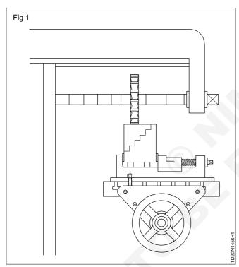
Mount the long arbor and the side and face milling cutter.
