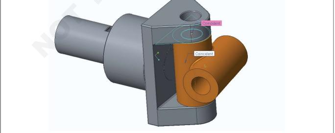
**Step 16:** Next repeat the step 3 to open the next component Pin. In component reference select the coincide option. This is done by selecting the cylindrical
