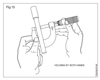
High skill is needed for obtaining accurate measurement with the outside micrometer. A wrong setting of the micrometer over the workpiece may cause,
