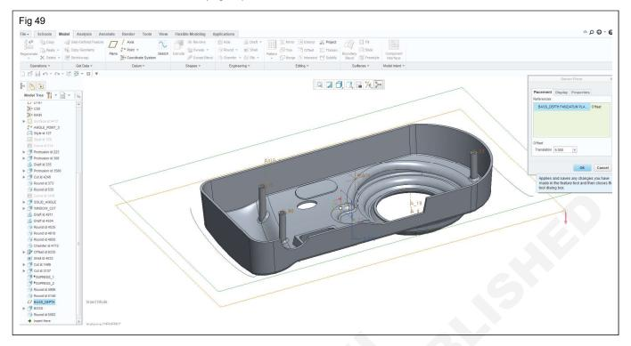
**Step 50:** Create the profile / Sketch for Ribs (Fig 50) extrude the profile upto the next surface.
