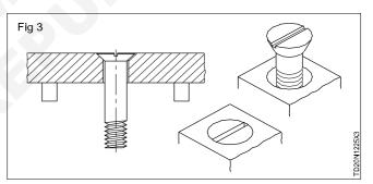
Check the countersink hole with a suitable countersink head screw for proper seating. (Fig 4)
