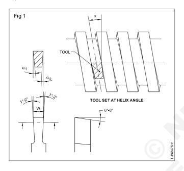
Helix angle =  $\tan^{-1} x \frac{\text{lead}}{\pi \times \text{core diameter}}$  and a<sub>2</sub> = Helix angle of the thread - 1°
