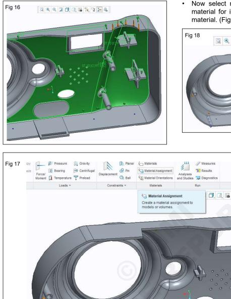
Now select material assignment in materials tab, material for individual volume and assign steel as material. (Fig 17, 18)
