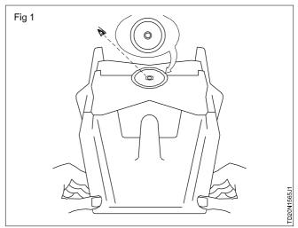
• Adjust the unit, using two knurled Screws on the base until the bubble in the levelling plate is concentric with the circle engraved on the glass.
