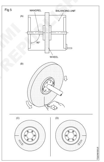
If the wheel finds the heavy points quickly, the balancing weights could be moved approximately 180°. (This indicates that the wheel is considerably out of balance). Move the weights equally towards the lighter side, approximately 3 mm at a time. Fig 6)
