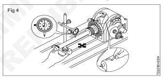
Rotate the head manually to ensure the bar is running true. Take a reading with the dial indicator as near the spindle nose as possible. (Fig 5)-A
