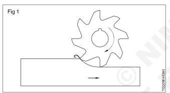
In up-milling the removal of chip by each cutting edge starts at the thinnest part of the chip (a) and progresses to the thickest part. (Fig 2) The cutting edge slides in the material before it starts to cut. This scraping
