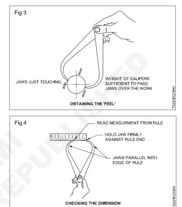
The point of one jaw must be placed over the graduation so that the point of the other jaw is parallel with the edge of the steel rule.
