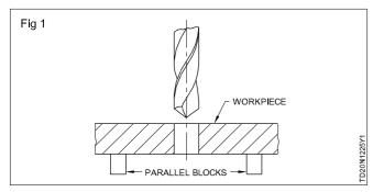
Set the location of the drilled hole position using the correct diameter drills.
