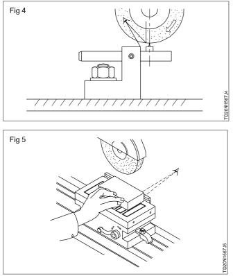
Set the table traverse-stopper dog considering the (Fig 6) approach length and over travel. Also set for the clearance of the job width.
