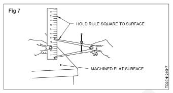
Read the graduation to an accuracy of +0.5 mm.
