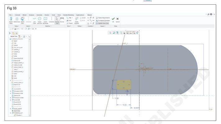
**Step 35:** Create the draft angle to the rectangle, extrude cut feature by selecting the bottom face (Fig 34, 35). In
