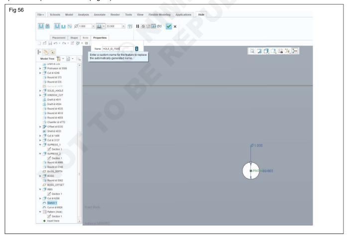
**Step 54:** Fill the sketched area with pattern member, space the member in the diamond pattern with value as 3mm (Set the distance any pattern members center can
