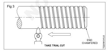
At the end of the trial cut, withdraw the tool immediately, winding it clear off the workpiece by operating the crossslide hand wheel and simultaneously reversing the machine. (Fig 4)
