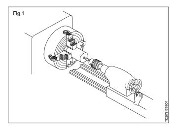
Mount a suitable centre drill securely in the drill chuck.
