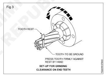
Tooth rest should support the peripheral tooth edge as close as possible to the edge of the end tooth.
