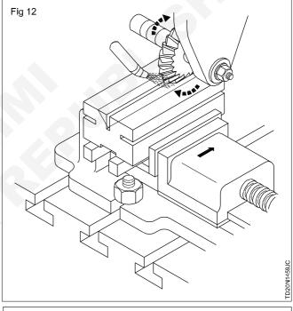
Apply automatic feed if your machine permits. If not, apply manual feed.
