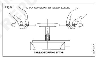
Continue cutting the thread. Turn backwards frequently about quarter turn, to break the chips. (Fig 7)
