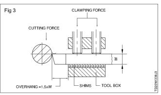
Tighten the tool with the centre screw of the tool post.
