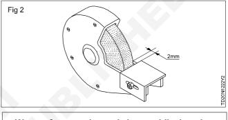
Wear safety goggles and gloves while dressing a grinding wheel. Stand on one side of the grinder while starting. Hold the dresser firmly while dressing. Do not put excessive pressure on the grinding wheels.
