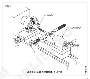
Remove the reamer occasionally by turning it clockwise to clear of the chips from the flutes.
