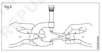
Note the readings on the barrel and thimble of the outside micrometer, and determine the size of the measurement.
