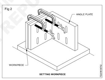
Clamp the work securely to the angle plate and set the clamps, so that they will not interfere with the grinding operation (Fig 3)
