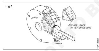
Switch on the grinder but stand by the side of the wheel for safety, and see whether the wheel runs 'true' and has no excessive vibration. In case of excessive vibration turning is necessary. Ask the instructor for advice.
