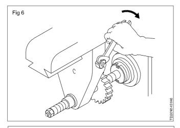
Ensure that the bearing bush extends equally on both sides of the arbor for uniform support.
