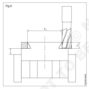
Mount the dovetail cutter in the collet chuck and tighten. Calculate and set the r.p.m. and feed for the dovetail cutter. Set the datum at the bottom surface of the step and the vertical face of the step, using tissue paper.
