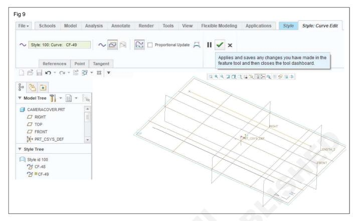
**Step 15:** Create another two datum points with curve F10 as point reference & to the offset distance as 30mm with offset reference as length\_2 plane (PNT 13) & (PNT
