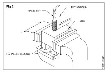
Fix the first tap (taper tap) in the correct size tap wrench. Too small a wrench will need a greater force to turn the tap. Very large and heavy wrenches will not give the 'feel' required to turn the tap as it cuts and may lead to breakage of the tap.
