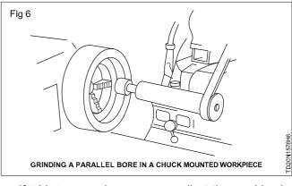
If table traverse is necessary, adjust the machine by setting the table reversing dogs.
