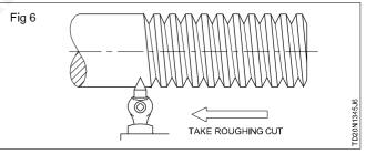
Use plenty of coolant during threading.
