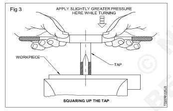
Remove the wrench from the tap when you are sure of starting the thread without disturbing the setting.
