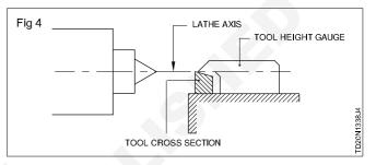
Remove or add shims and check the height when the tool is tightened by the centre screw.
