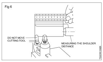
Turn the carriage hand wheel to move the cutting tool away from the shoulder slightly.
