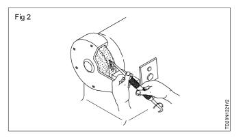
For grinding the point hold the scriber vertically on the grinding wheel face and rotate it with the fingers.
