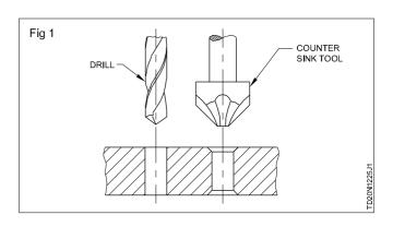
Remove the centre dill, hole the twist drill of the required dia. Check if it 'runs true'. Start drilling the through hole.
