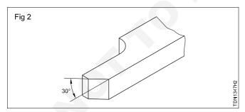
Repeat the above procedure on the right side of the tool to get an included angle of 60 on the tool (Fig 3)
