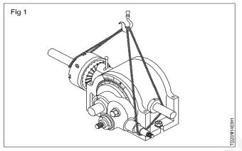
Lift the indexing head with help of crane and position it on the milling machine table.
