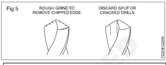
Never re-sharpen a cracked or split drill. Avoid overheating the drill.
