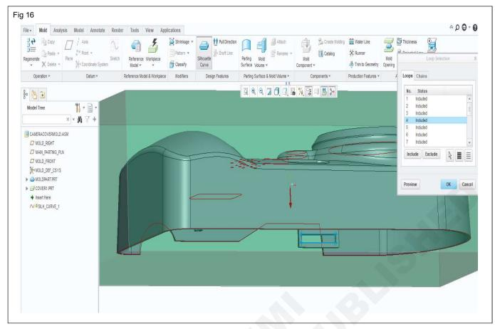
**Step 21:** Select Mold volume  $\rightarrow$  Mold volume then select Extrude  $\rightarrow$  in placement tab select define, sketch
