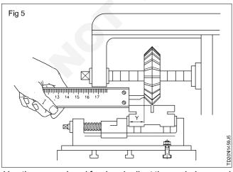
Use the cross - hand feed and adjust the workpiece such that the cutter surface and the workpiece edge are at [Y] distance.
