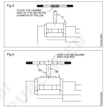
Cut thread slowly and reverse the die for a short distance in order to break the chips.
