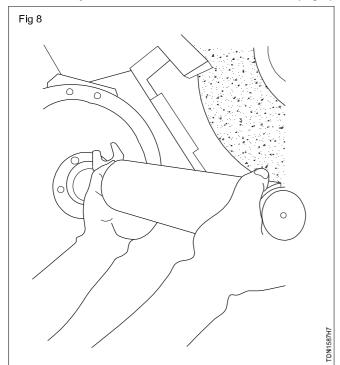
Hold the work with the left hand as illustrated while holding the work to prevent the centre hole coming out.
