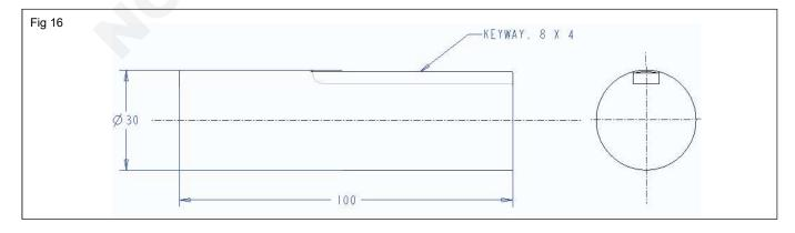
• Sketch the solid shaft with keyway as shown in Fig 17.
