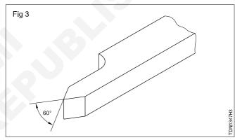
Check the tool by centre gauge, there should not be any right passing through gauge and cutting edge of the tool.
