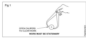
Place one point of the leg over the workpiece and get the sense of feel of the other point of the leg.
