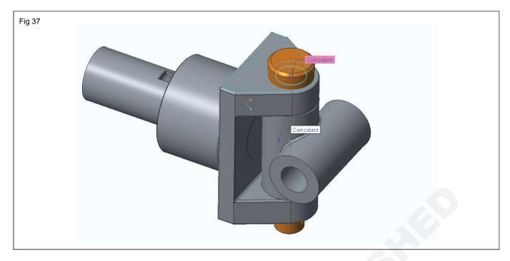
**Step 18:** Select / Insert collar by repeating the step 3 Select the cylindrical face of collar and cylindrical face of pin-select coincide as component mate reference and select coincide of axis for collar taper pin hole to pin-taper pin hole. (Fig 38). Click v ok option.
