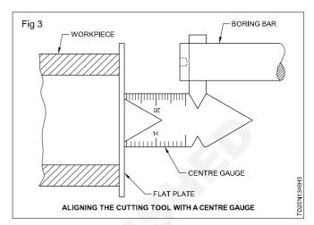
Mark the boring bar to indicate the required depth of entry into the bore.
