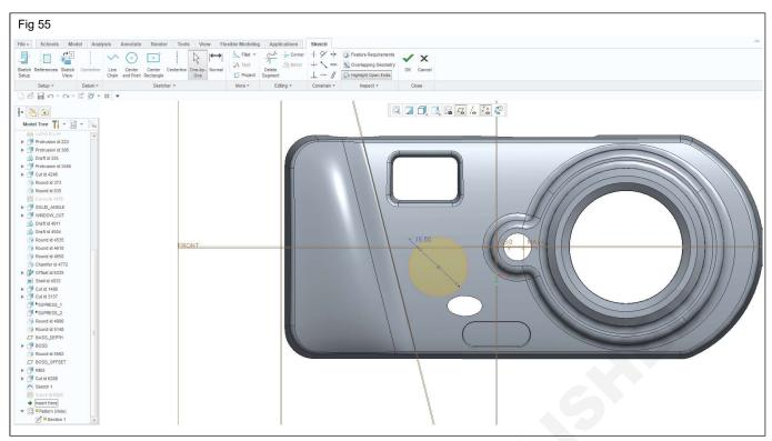
Select create simple hole use predefined circle as drill hole profile with  $\phi 1$  drill from placement ref. by a specified depth value as 33. (Fig 56)
