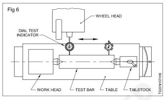
Fix the test bar in between centres.
