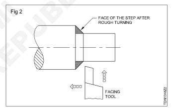
Make sure that the tool bit is set up with the point close to the work, and with a slight space along the side cutting edge.
