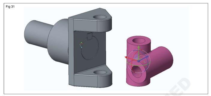
Step 15: Select the interior hole face of centre block and fork hole cylindrical face to coincide and then
