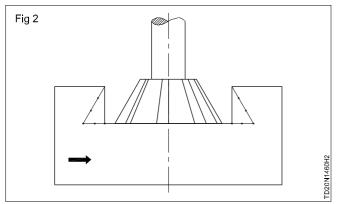
Set the datum at the vertical face of the slot by touching the edge of the dovetail cutter. (Fig 3)
