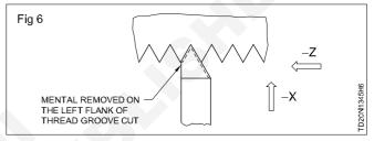
Continue the sequence till the thread profile is formed. (Fig 7)
