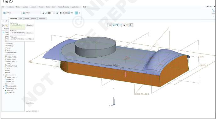
**Step 30:** Draw another circle on the top plane with ø 48.88 & extrude the sketch to about 8mm, place by a specified depth value option. (Fig 29)
