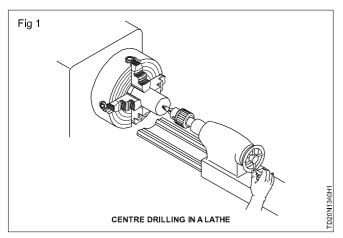
Select the required size drill and hold the drill in the tailstock spindle sleeve/ drill chuck.
