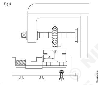
Measure the thickness of the cutter (T).
