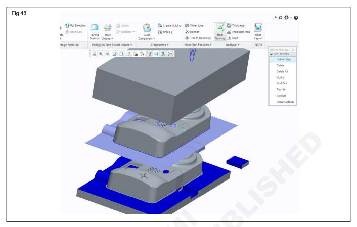
**Step 40:** Once again click the mold opening, the parts are moved as per the given direction by us (Fig 49,50&51).
