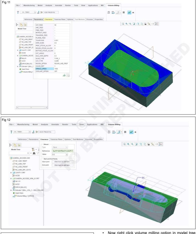
Note: In order to view machinery process in cavity we are hiding work piece & mill volume. • Now right click volume milling option in model tree then select play path.
